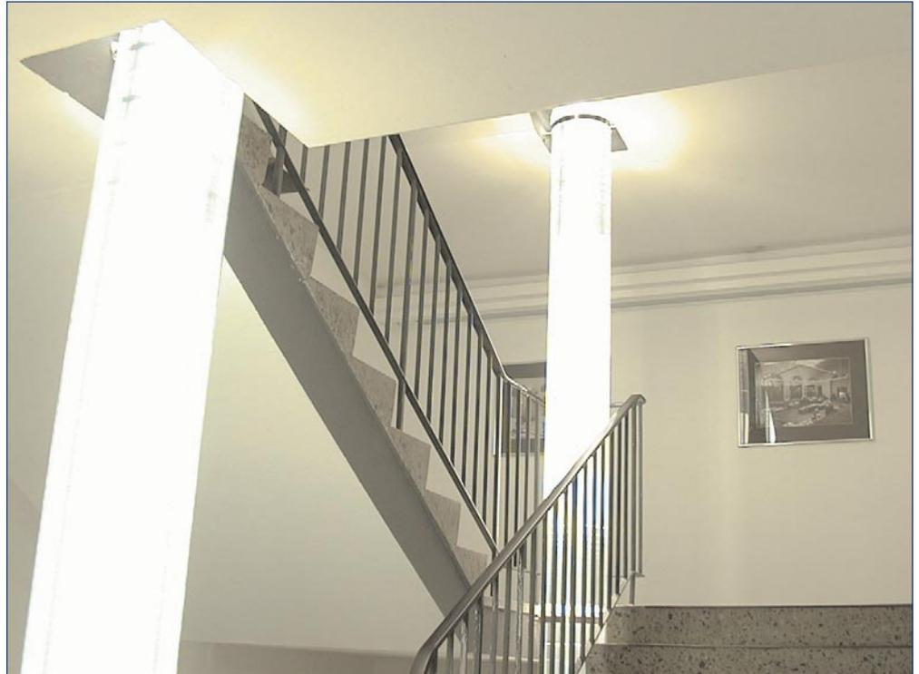
Hollow Light Guide System - Berlin Prototype at Semperlux
